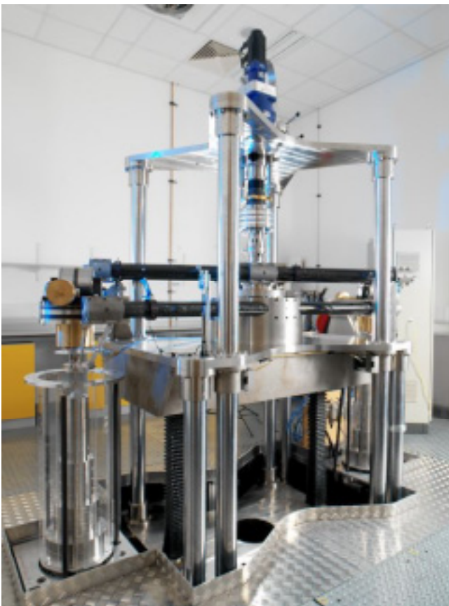
Fig. 4. NPL 2 kN·m machine.
