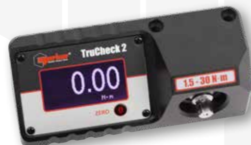
30 N-m model showing horizontally aligned male hexagon
